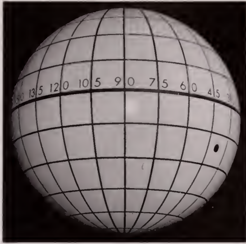
FIG. 2. Having determined the spherical coordinates of the gradient, it is represented by a spot on the surface of a sphere.
