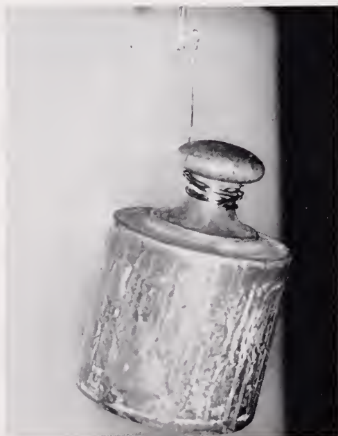
FIG. 3. Eight-ounce weight suspended from the neck of the stapes indicates the amount of force which the neck of some stapes can withstand without fracture of the crura.
